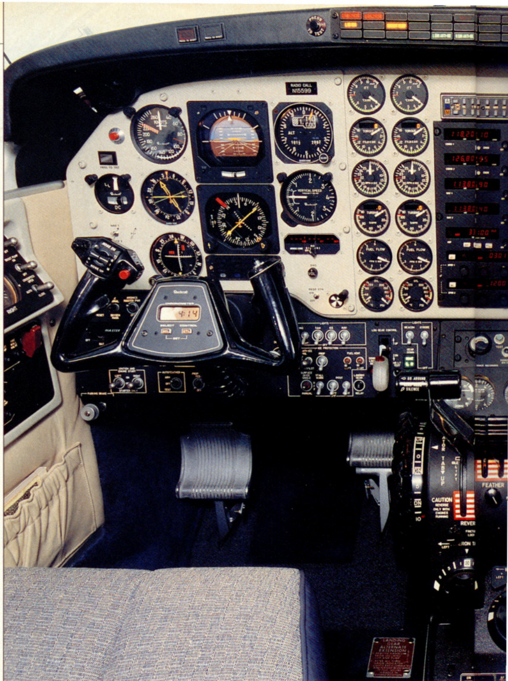
Electro-mechanical instruments and panel-mount avionics differentiate the C90SE panel from its more expensive sibling, the C90B (below), which uses EFIS and remote-mount avionics. Interior fabrics, leathers, and color choices are the same for either model, but the SE comes standard with four instead of six cabin seats (right).
