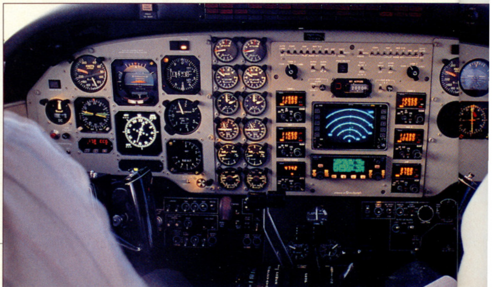
Electro-mechanical instruments and panel-mount avionics differentiate the C90SE panel from its more expensive sibling, the C90B (below), which uses EFIS and remote-mount avionics. Interior fabrics, leathers, and color choices are the same for either model, but the SE comes standard with four instead of six cabin seats (right).
